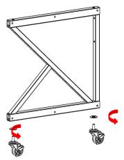
Step 2: Thread each caster all the way in to the insert so that no threads are exposed.
