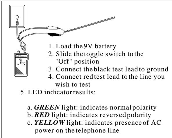
**Note:** If a ground is not available, you may try to switch the test leads around to different wires within the pair. The LED indicator will light GREEN when the red test lead is connected to the ring side of the line and the black lead is connected to the ground.
