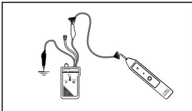
4. Select either a dual alternating tone or a single solid tone by positioning the button on the face of the Tone Generator unit to "DUAL TONE" or "SINGLE TONE."
