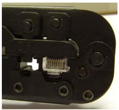
The last step is to actually crimp the connector. You may be asking "So what's actually happening during the crimping process?"
