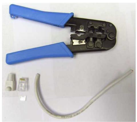
Step 1: Slide on the Strain-Relief Boot
