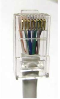
Step 5: Trimming the Cable and Slipping the Connector on the Cable
