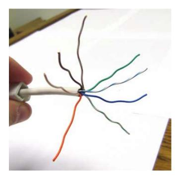
There are a few different orders the wires can go in depending on the application you're using this cable for. The most common standards are T568A and T568B. T568A is the recommended wiring standard according to the ANSI/TIA/EIA. T568B is the older and more widely used of the two standards. The main difference between the two is that the orange and green pairs of wires are switched, however, it's important to note in terms of functionality they accomplish the same thing.
