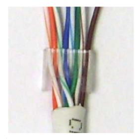
Step 4b: Cutting the Wires (Without Insert)
