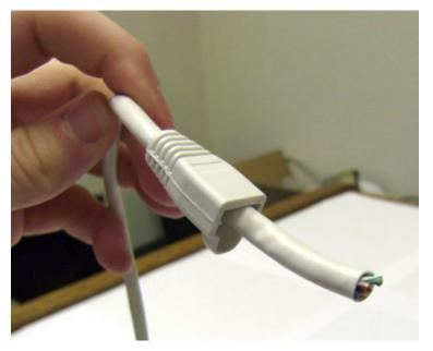
The first step we will perform is to slide on the strain-relief boot. This is done by slipping the cable through the hole in the boot. You will want to make sure the larger side of the boot (the part that the plastic connector will sit in) is facing towards the end of the cable. Strain-relief boot are optional, they are used to keep the wires from being bent at too sharp an angle after coming out of the connector.
