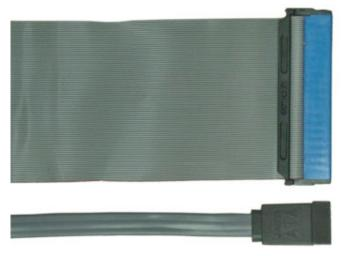
The narrow design of the Serial ATA cable allows for more flexibility in running the cable, as well as improved airflow within the computer.
