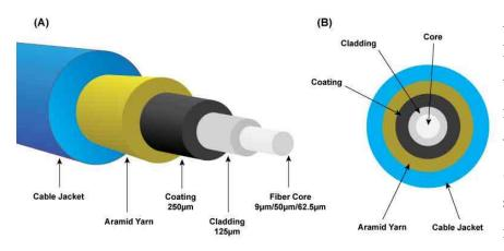
As we progress through the history of fiber optics, we see that during the early 1970s multimode fiber was very influential, with variants of 62.5 microns and 50 microns. The inception of single-mode fiber with an 8.3micron diameter core marked a
