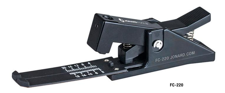
Designed to cleave either 900µm buffered or 250µm coated fiber, this fiber cleaver's quick and easy three step operation is perfectly suited for mechanical splicing and quick field termination of fiber connectors. This fiber cleaver features the following:
